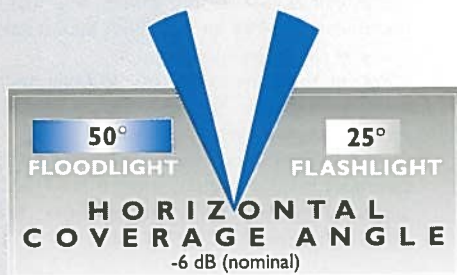
Floodlight delivers a 50° horizontal coverage pattern.
