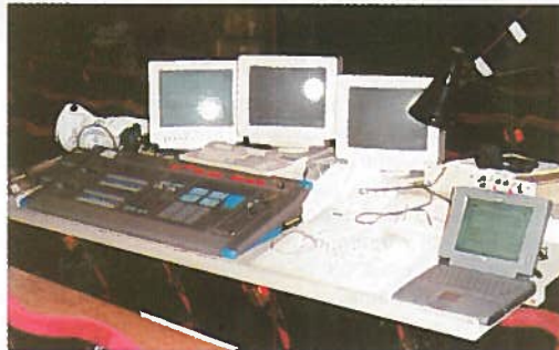
Moving light control - Arri Imagine 3, Apple Macintosh for the DLCs, Powerbook for keeping track of everything - in the stalls during the production period.
