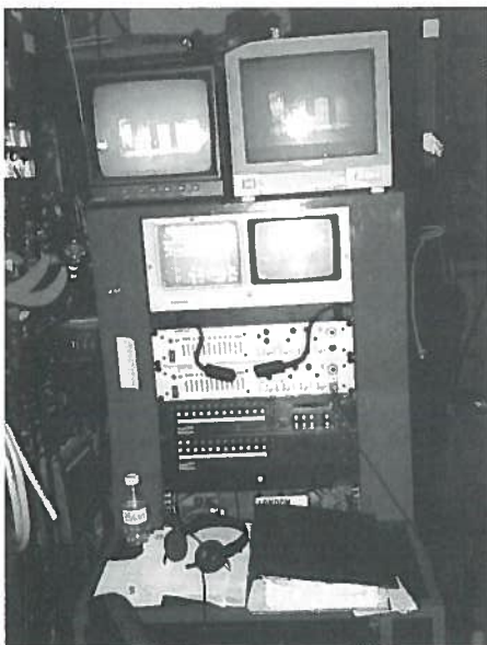
The Soft-Cue computerised prompt desk system supplied by Howard Eaton Lighting.
