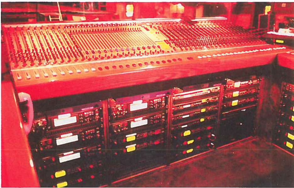
The heart of the sound system - a 92-channel Cadac J-type desk, one of the largest of its kind, and the first to feature the 'flying fader' system.
